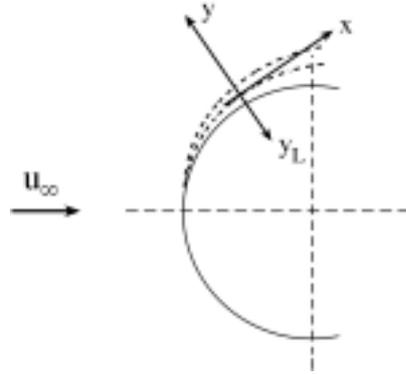
Fig.1 The double boundary layer and the Cartesian coordinates.
