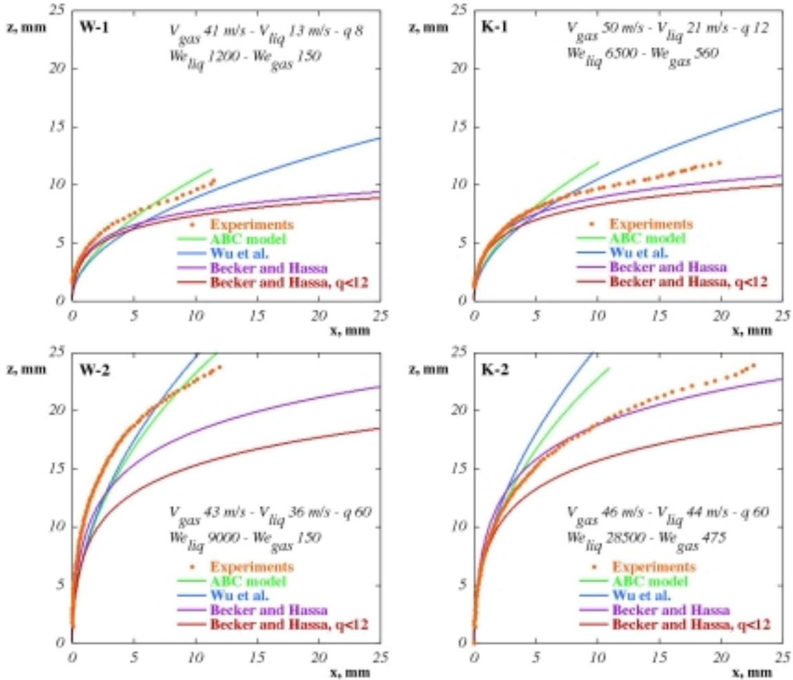
Fig. 2 Comparison between experimental spray windward profiles and trajectories predicted by the ABC model and other model from literature
