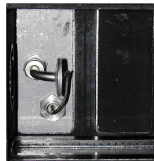
Figure 5. FLAMESEEK flame stabilizer; flow is left to right.
