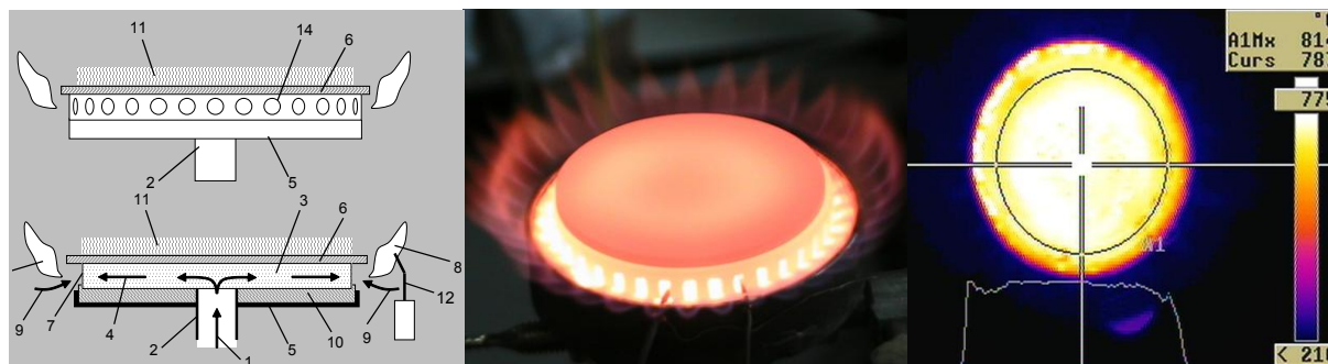
Fig. 1 Schematic drawings of the novel catalytic hybrid cooktop burner and images of the prototype developed and operated at IRC. The InfraRed picture shows the high temperature radiating cap of the burner.
