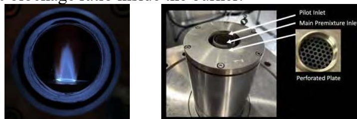
Figure 1. a. The turbulent premixed flame of 0.8 equivalence ratio with no hydrogen addition. b. The burner.
