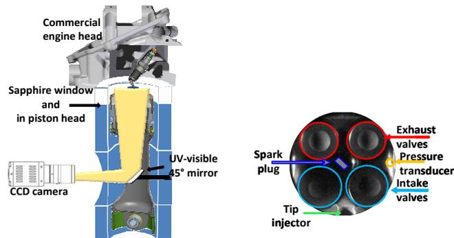
**Figure 1.** Optical setup and field of view of the combustion chamber.
