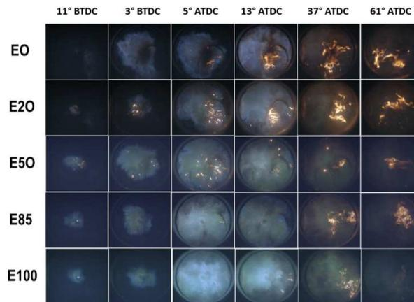
**Figure 2.** Selection of combustion frames for the tested fuels at 2000 rpm full load.
