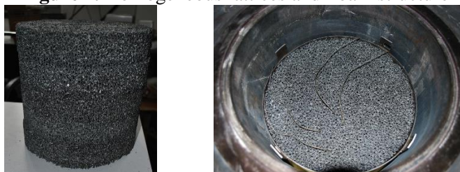
Figure 3. Coated conventional foam a) without canister and b) into the ATR unit
