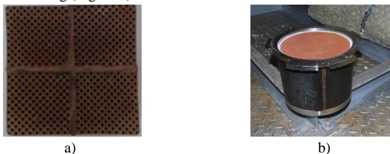
Figure 3. a) Monolithic assemblies consisting of 4 smaller monoliths for the pilot scale experiments and b) coated filter for the demonstration plant.
