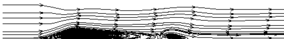
Figure 8. Flow field with incident shock wave introduced upstream of the injector
