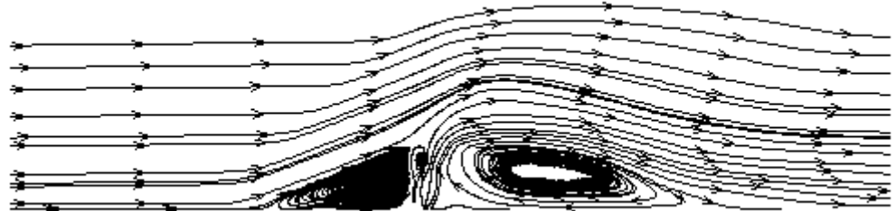
Figure 11. Flow field with incident shock wave introduced downstream of the injector
