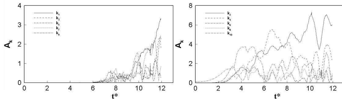
**Figure 7.** Amplitude of the flame front cells at different wave numbers as a function of time. The initial pressure is 25 atm and initial wave number is 6.
