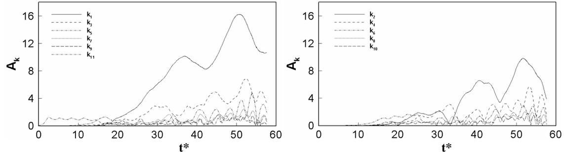
**Figure 4.** Amplitude of the flame front cells at different wave numbers as a function of time. The initial pressure is 5 atm; the initial disturbance at the flame front has a wave number of 11.
