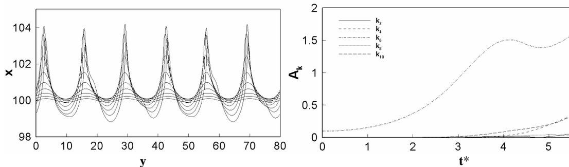
**Figure 2.** (a) Evolution of the flame front at the linear growth period, (b) amplitude of the flame front cells at different wave numbers as a function of time. The initial pressure is 5 atm; the initial disturbance at the flame front has a wave number of 6.
