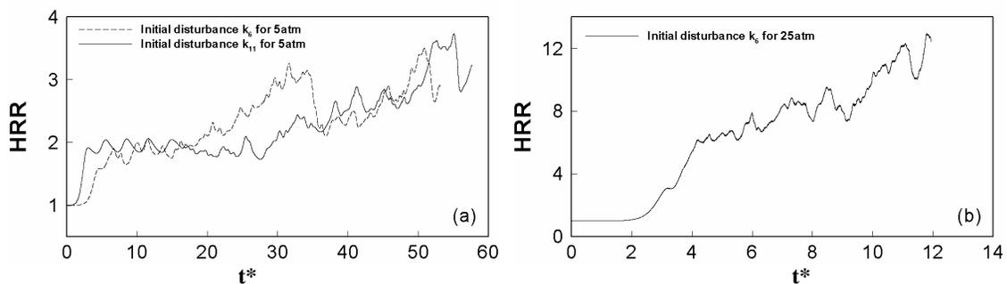
**Figure 5.** Total heat release rate (volume integrated in the entire domain) as a function of time. (a) case A, (b) case B. The heat release rate for each is normalized by its corresponding one in the planar flames.
