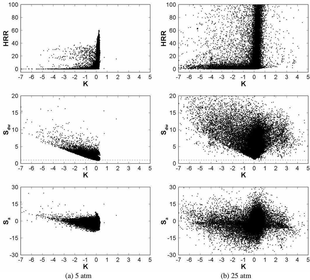
**Figure 8.** Scattering of heat release rate, density-weighted displacement speed and absolute normal flame speed as functions of curvature for (a),  $20 < t^* < 53$ , case A, and (b)  $8.5 < t^* < 12.95$ , case B.
