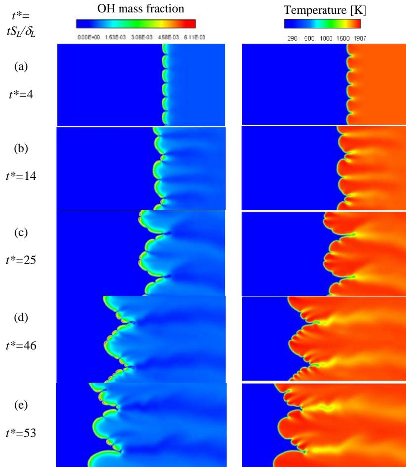
**Figure 1.** Instantaneous field of OH mass fraction and temperature showing five critical instances of time for case A. (a) at the end of the linear growth stage, (b) at the instance that larger cells with  $k=2$  become dominant, (c) at the instance that cells with odd wave number appear, (d) at the instance that cells with odd wave number start to grow rapidly.
