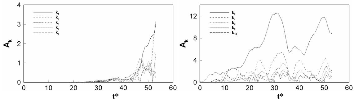
**Figure 3.** Amplitude of the flame front cells at different wave numbers as a function of time. The initial pressure is 5 atm; the initial disturbance at the flame front has a wave number of 6.
