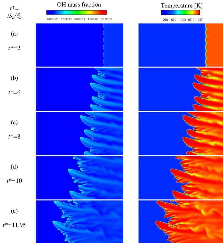
**Figure 6.** Instantaneous field of OH mass fraction and temperature showing five critical instances of time for case B. (a) at the end of the linear growth stage, (b) at the instance that odd number of wave cells appear, (c) at the instance that the amplitude of  $k_2$  cells become the largest, (d) at the instance that cells with odd wave number grow rapidly.
