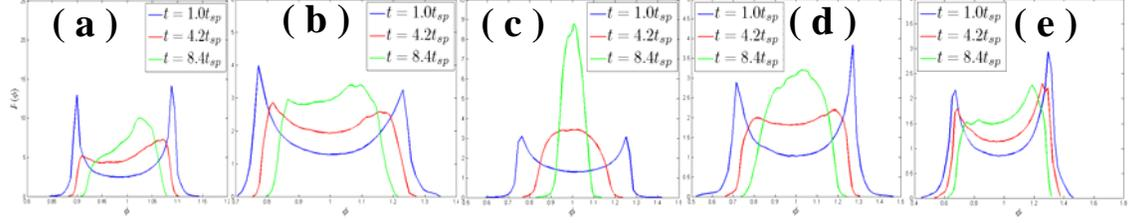
**Figure 5** Temporal evolution of the PDFs of equivalence ratio  $\phi$  at  $t = 1.0t_{sp}$ ,  $t = 4.2t_{sp}$  and  $t = 8.40t_{sp}$  for cases (a) D, (b) G, (c) H, (d) I and (e) J.
