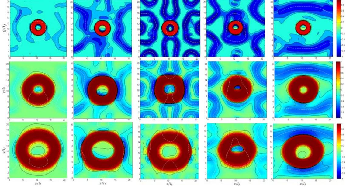
**Figure 4** The distributions of  $I_c = \nabla Y_F \cdot \nabla Y_0 / |\nabla Y_F| |\nabla Y_0|$  at the central  $x_1$ - $x_2$  plane for cases D [Column 1], G [Column 2], H [Column 3], I [Column 4] and J [Column 5] at times  $t = 1.0t_{sp}$  [Row 1],  $t = 4.20t_{sp}$  [Row 2] and  $t = 8.40t_{sp}$  [Row 3].
