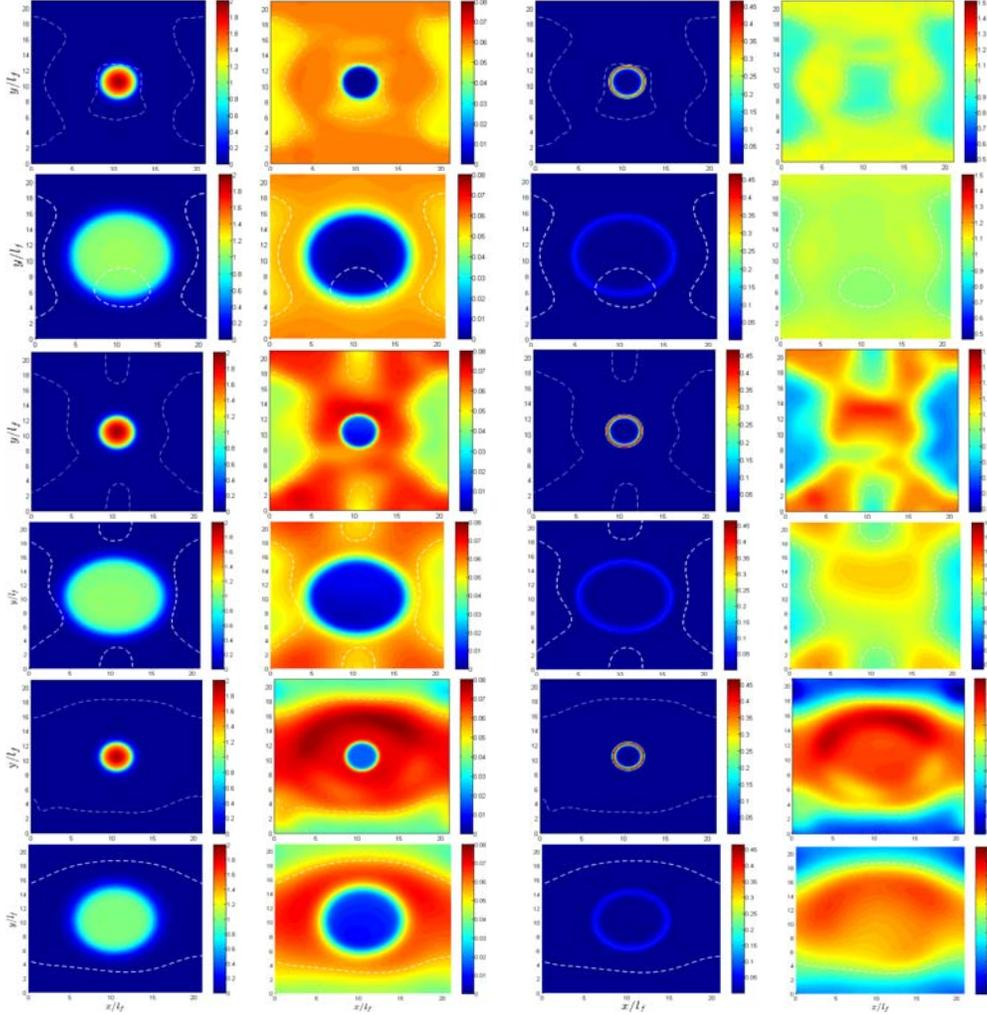
**Figure 2** The distributions of  $T$  [Column 1],  $Y_F$  [Column 2],  $\dot{w}_F \times l_f / \rho_0 S_{b(\phi=1)}$  [Column 3] and  $\phi$  [Column 4] at  $t = 1.0t_{sp}$ ,  $8.40t_{sp}$  [Rows 1-2 for case D], [Rows 3-4 for case G] and [Rows 5-6 for case J] at the central  $x_1$ - $x_2$  plane. The white line indicates the  $\xi = \xi_{st}$  contour.
