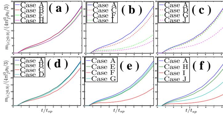
**Figure 8** The temporal evolutions of the burned gas mass normalised by the mass of unburned gas with radius equal to  $l_f$  (i.e.  $4/3\rho_0\pi l_f^3$ )  $m_b(c \geq 0.9)/(4/3\rho_0\pi l_f^3)$  for cases (a) A, B, E and H, (b) A, C, F and I, (c) A, D, G and J, (d) A-D, (e) A and E-G, and (f) A and H-J.
