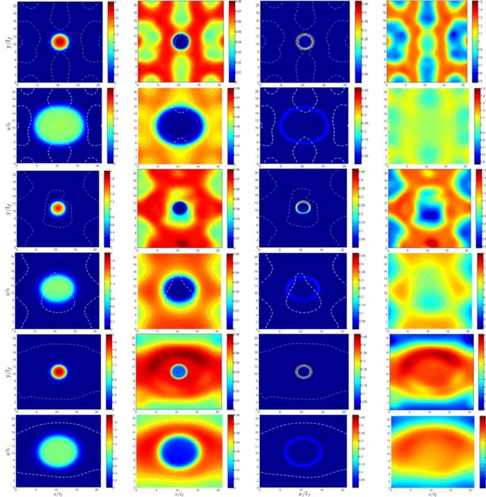
**Figure 3** The distributions of  $T$  [Column 1],  $Y_F$  [Column 2],  $\dot{w}_F \times I_f / \rho_0 S_b(\phi=1)$  [Column 3] and the equivalence ratio ( $\phi$ ) [Column 4] at  $t = 1.0t_{sp}$ ,  $8.40t_{sp}$  [Rows 1-2 for case H], [Rows 3-4 for case I] and [Rows 5-6 for case J] at the central  $x_1$ - $x_2$  plane. The white line indicates the  $\xi = \xi_{st}$  contour.
