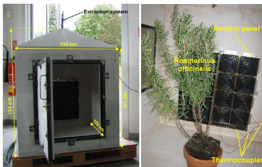
Figure 1. Pictures of the VOCs emissions experimental setup.
