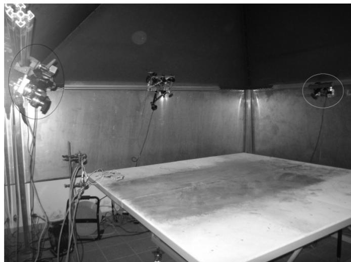
**Figure 2.** Stereovision cameras positioned in a front position and in a back position relative to the direction of the fire propagation
