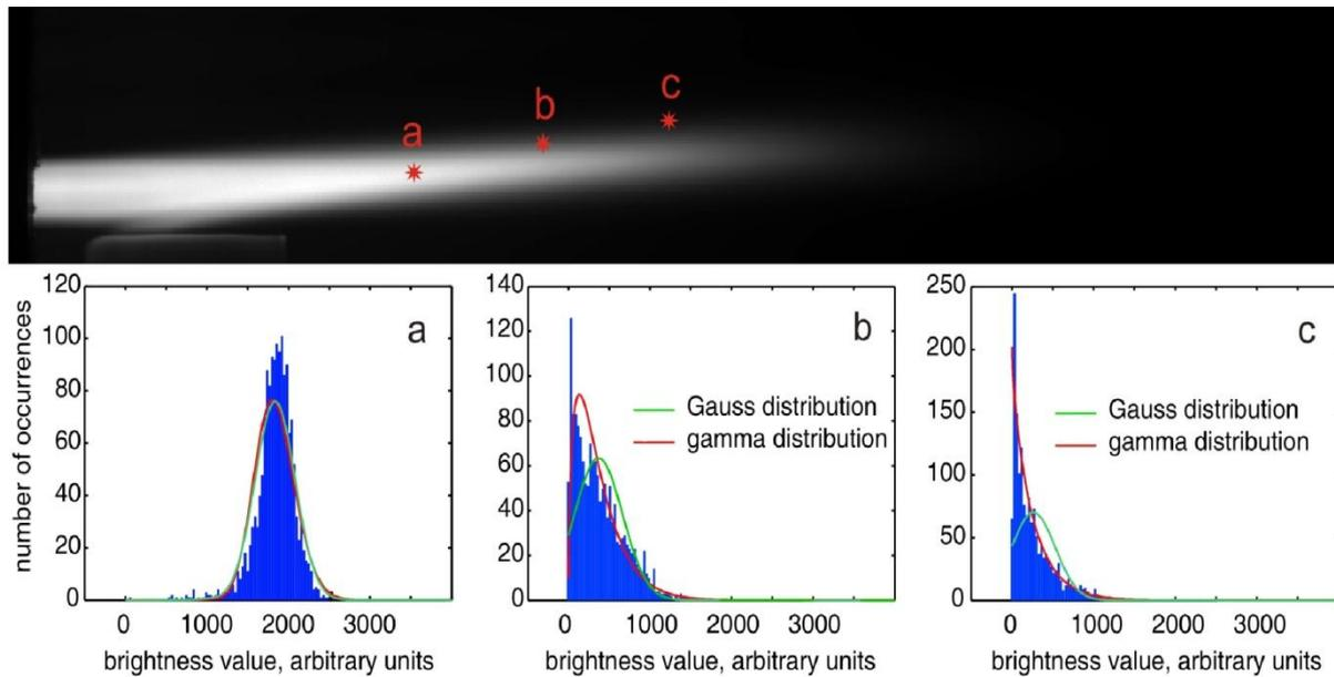
**Figure 5.** Brightness distribution shapes in different locations of plasma jet (a-centre of the jet, b-fringes, c-far fringes).
