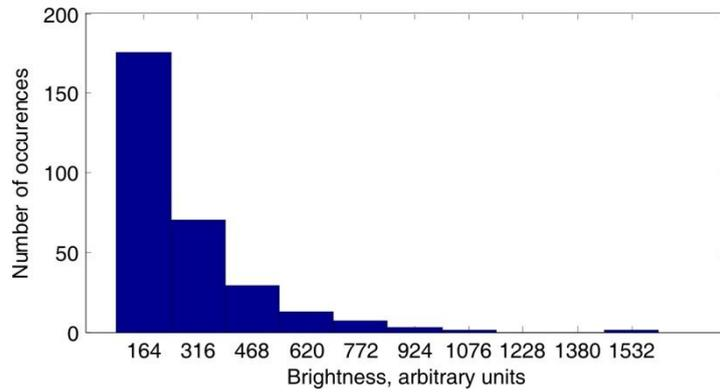
**Figure 6.** Histogram of brightness distribution in the fringe of plasma jet.
