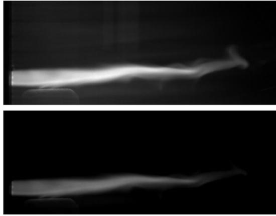
**Figure 2.** Views of the same plasma jet with different sensitivities of optical system (diameter at the nozzle exit is 6 mm).
