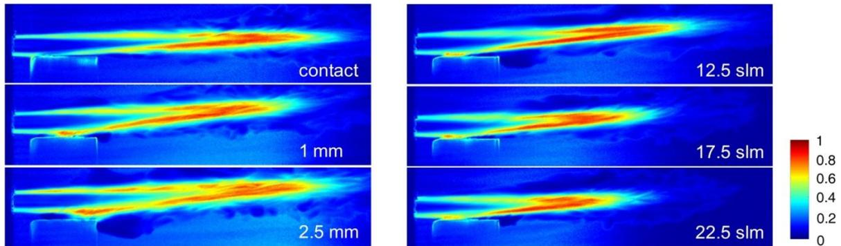
**Figure 7.** Maps of relative entropy of plasma jet in dependence on anode surface distance from the jet (left) and in dependence on argon flow rate (right).
