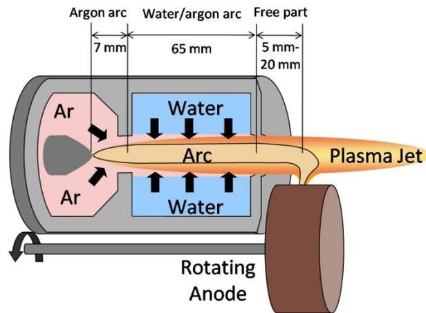
**Figure 1.** Schematics of thermal plasma torch with argon-water stabilization of arc.
